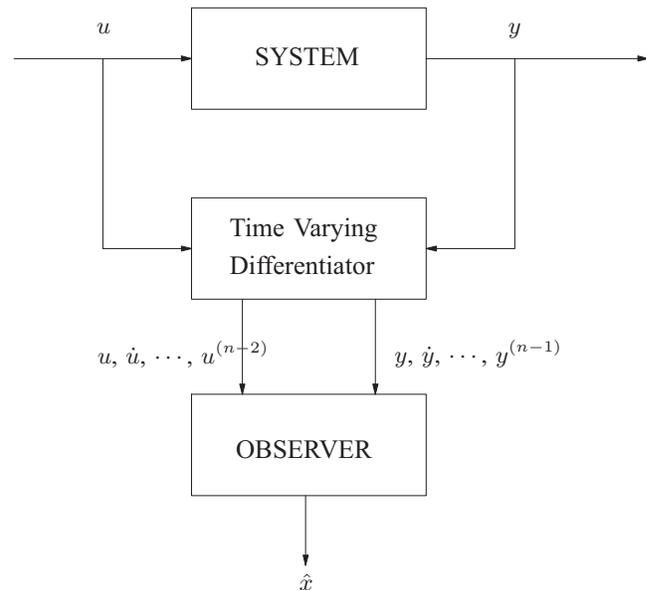
Fig. 1. The scheme of the nonlinear observer
