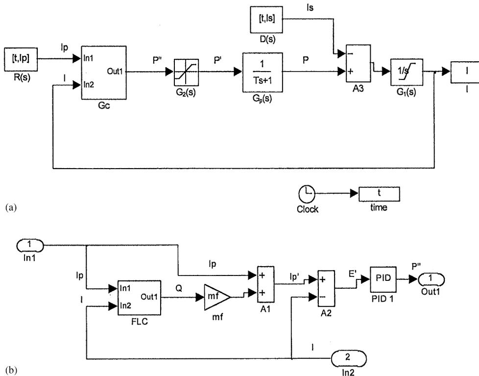
Fig. 1. Simulation model for production–inventory control system: (a) Overall system, (b) controller.
