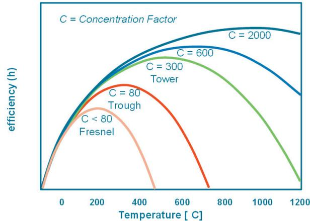
Fig. 1. Solar thermal plant efficiency variation with temperature
