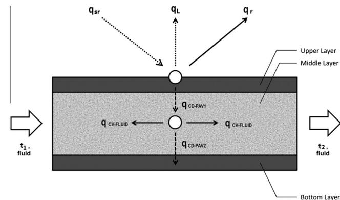
Fig. 1. Heat transfer process of pavement solar energy harvested [19].
