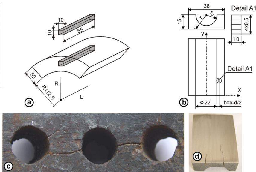
**Fig. 1.** Cutting scheme of specimens taken from perforated area of collector: (a) for testing on Charpy toughness; (b) for measurement of hardness and microhardness; (c) part of the 12Cr1MoV steel collector with holes for nozzles, (d) thin section for microstructural studies.
