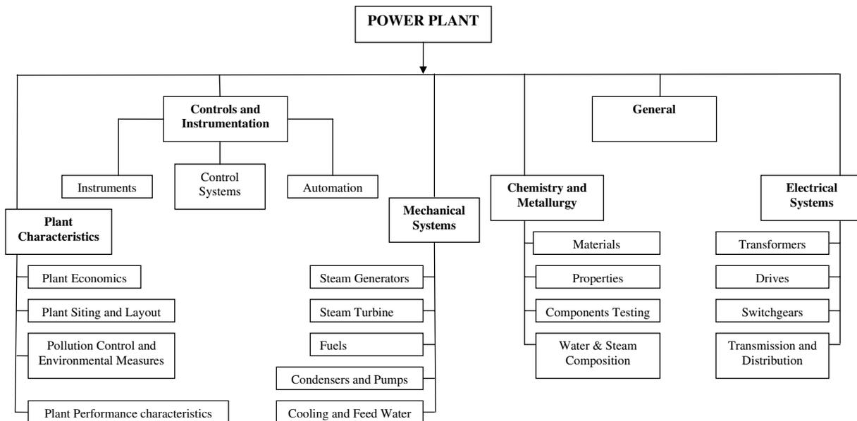
Fig. 1. Hierarchical structure of a fossil fired power plant.
