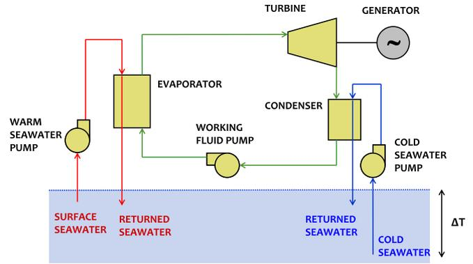
Fig. 3. Closed OTEC cycle.
