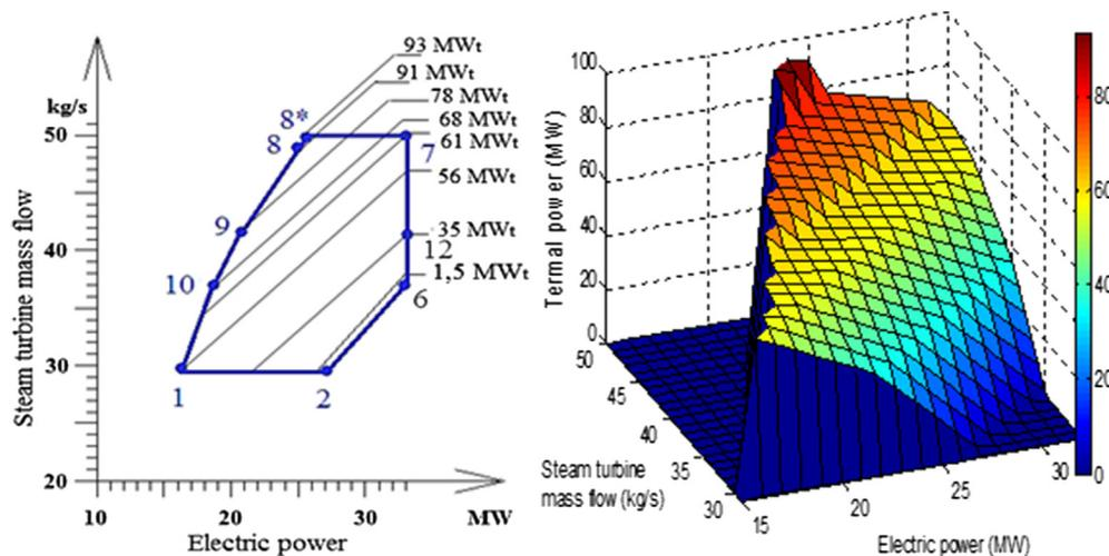
Fig. 1. Turbine real process production diagram [26].
