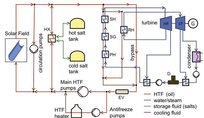
Fig. 2. Schematic diagram of a parabolic trough solar thermal power plant with thermal storage. In the figure, HX stands for heat exchanger, PH, SG, SH and RH for preheater, steam generator, superheater and reheater, respectively, D stands for deaerator and EV for expansion vessel.
