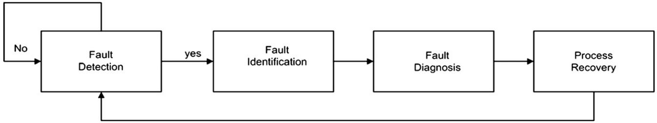
Fig. 1. A schema of the process monitoring loop [2].
