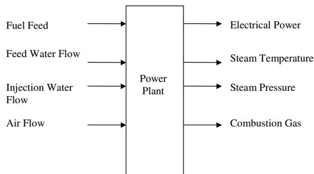
Fig. 1. Power plant as multivariable dynamic system.
