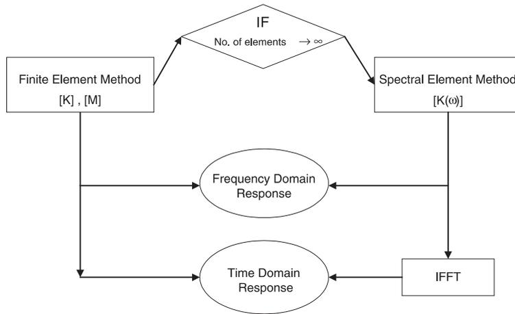
Fig. 1. Relations between FEM and SEM models.
