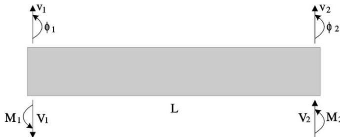
Fig. 2. Timoshenko beam with end loads and DOF.
