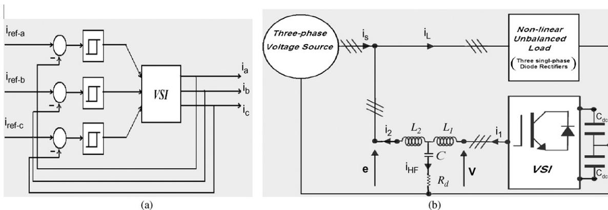
Fig. 1. (a) A typical current-control of a voltage-sourced inverter using the hysteresis modulation technique, (b) an active filter consists of an *LCL* passive filter that interconnects a VSI to the grid system.
