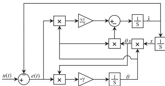
Fig. 1. Block diagram of the modified ANF.
