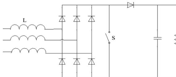
Fig. 2. the main circuit of three-phase single-switch PFC
