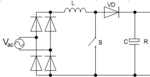
Fig. 1. the main circuit of single-phase single-switch PFC
