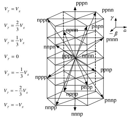
Fig. 3 Four-leg converter switching vectors in  $\alpha\beta\gamma$  coordinate space
