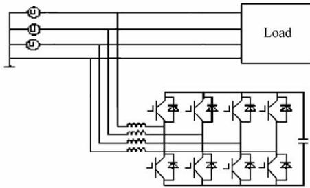
Fig. 1 Configuration of three-phase four-wire APF with four-leg converter
