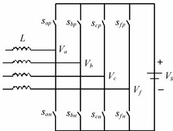
Fig. 2 Equivalent circuit of four-leg active filter
