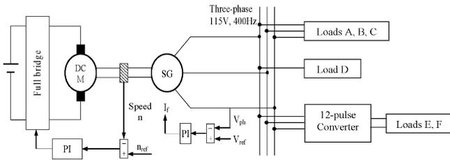
Fig. 1. Simulated structure for conventional aircraft electric power system.
