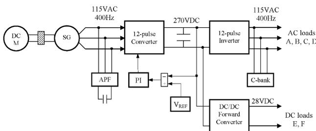
Fig. 2. Simulated structure for advanced aircraft electric power system.
