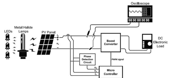
Fig. 1. Arrangement of PV power system.
