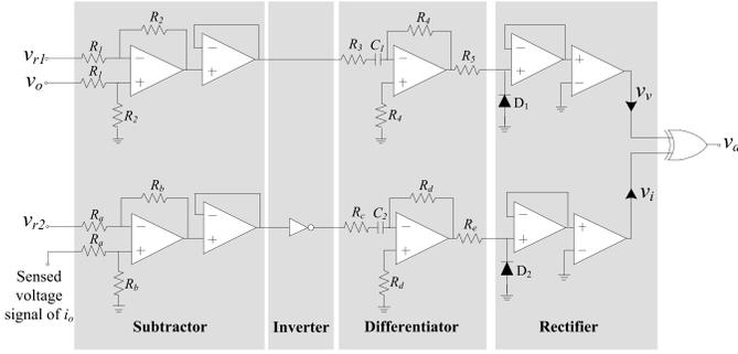
Fig. 2. Detection circuit of phase difference between PV voltage and current.
