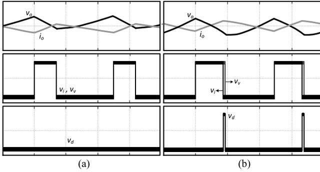
Fig. 3. Illustration of detective signal detection. (a)  $I_o < I_d$ . (b)  $I_o = I_d$ .
