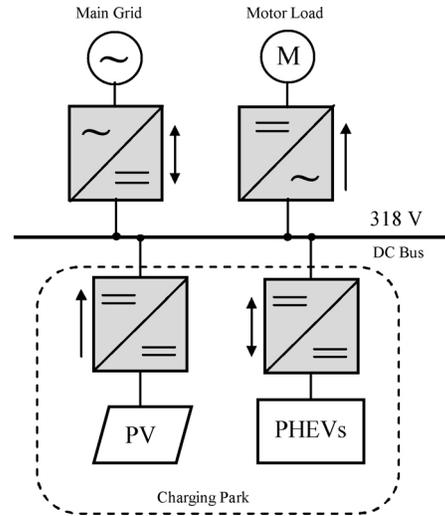
Fig. 1 Schematic diagram of the investigated system
