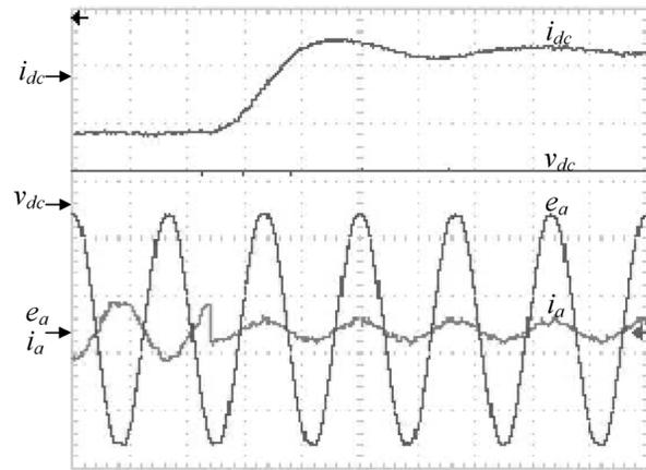
Fig. 2 Bi-directional converter response to a step change in the DC current reference from -4 to 1 A. (a) DC current,  $i_{dc}$  (4 A/div, 10 ms); (b) DC voltage,  $v_{dc}$  (1000 V/div, 10 ms); (c) AC phase voltage,  $e_a$  (30 V/div, 10 ms); (d) AC current,  $i_a$  (5 A/div, 10 ms).
