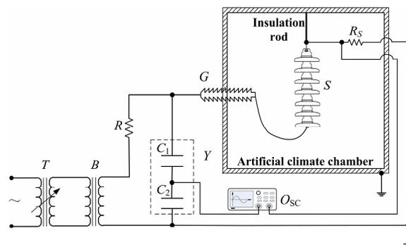
Figure 1. Schematic circuit of CEPRI chamber.
