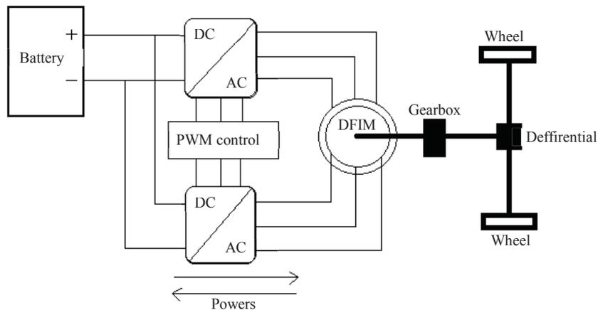
Fig (1): Representative diagram of the electric vehicle drive train
