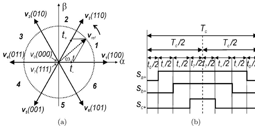
Fig. 1. Voltage space vectors and decomposition of the reference vector (a). Symmetrical switching pattern in sector 1 (b).
