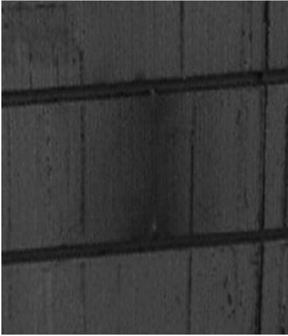
Fig. 1. A zoom of the damaged area due to interbar current.
