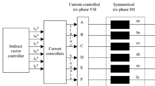
Fig. 1. Symmetrical six-phase vector controlled induction motor drive.
