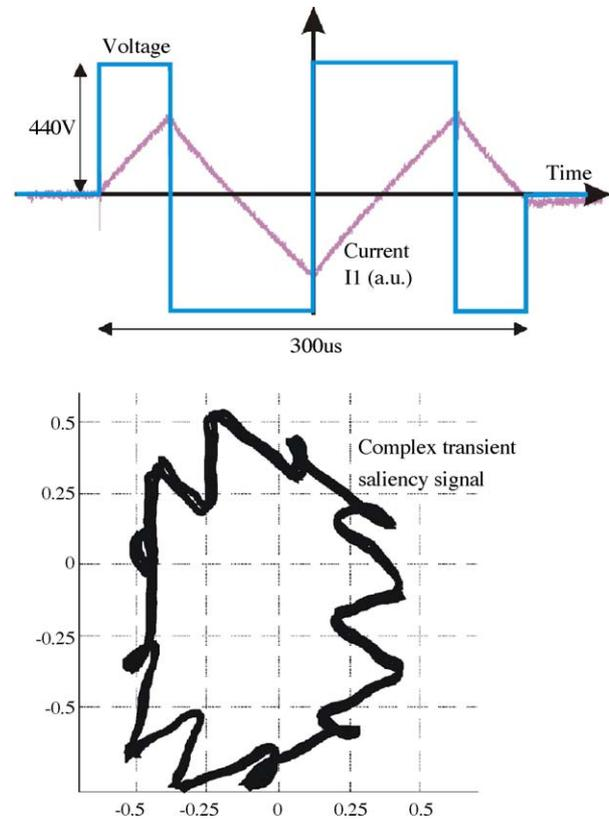
Fig. 1. (Upper) Injection signal and corresponding current response of the INFORM method; (lower) locus of the extracted saliency signal of a standard induction machine (complex plane; a.u.).
