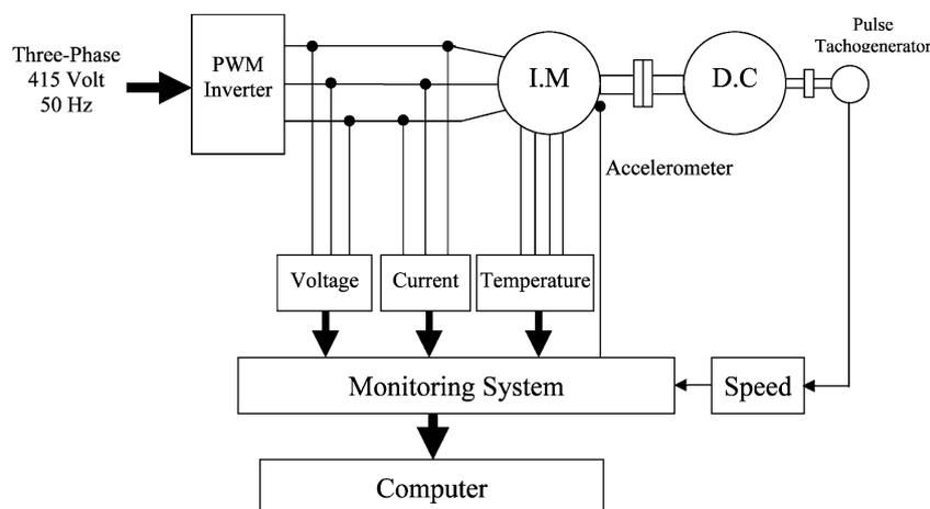
Fig. 1. Schematic diagram of the monitoring system.
