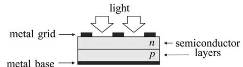
Fig. 1. Physical structure of a PV cell.
