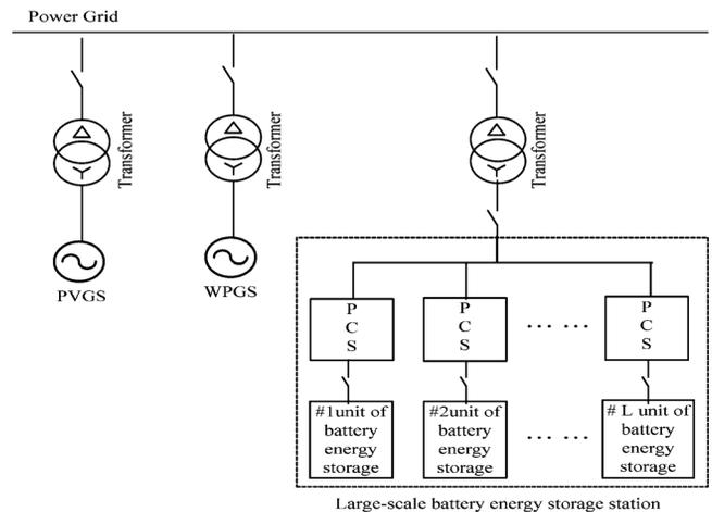
Fig. 1. Wind/PV/BESS hybrid power generation system.
