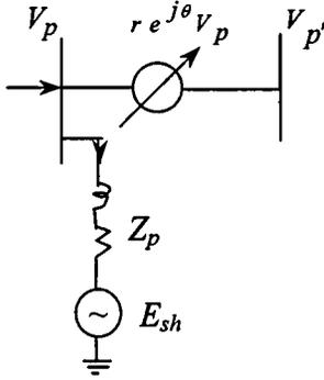
Fig. 2. Equivalent voltage representation of UPFC.
