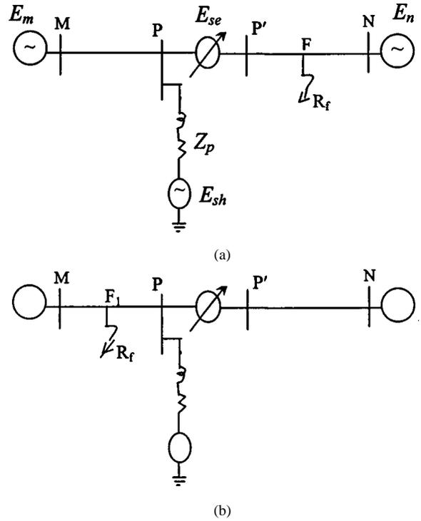
Fig. 3. (a) System under study for fault at  $F$  and (b) system under study for fault at  $F_1$ .
