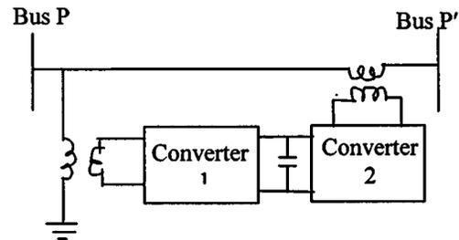
Fig. 1. Basic circuit arrangement of UPFC.
