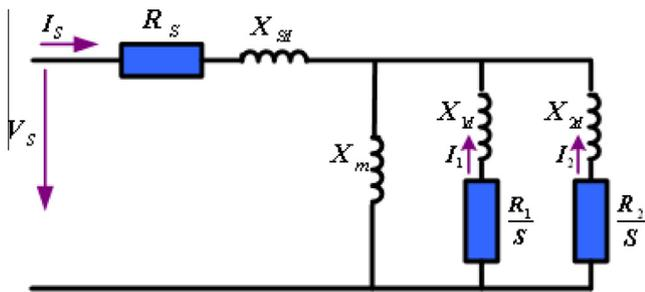
**Figure 2** Double-cage induction motor steady state model.
