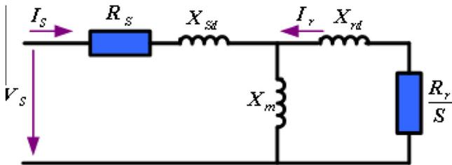
**Figure 1** Single-cage induction motor steady state model.
