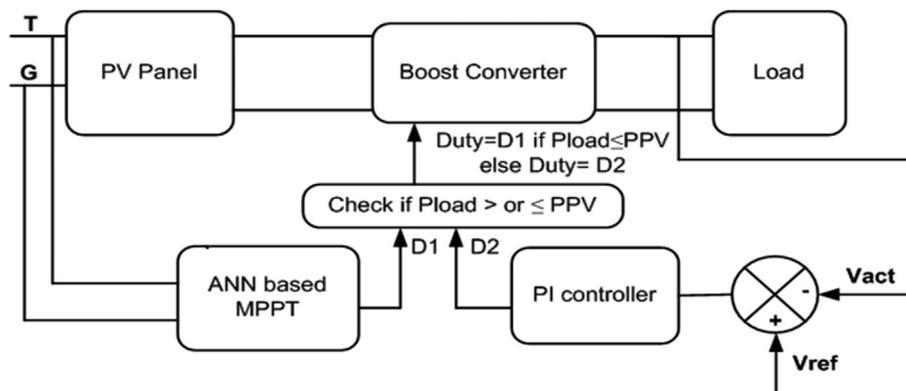
Fig. 1. PV system with ANN based MPPT.
