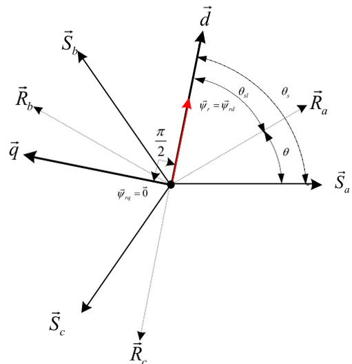
Fig. 1. Reference frame (d–q) orientation according to the rotor flux vector.
