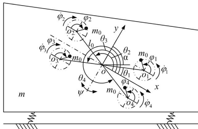
Fig. 1. Dynamic model of a linear vibratory feeder.
