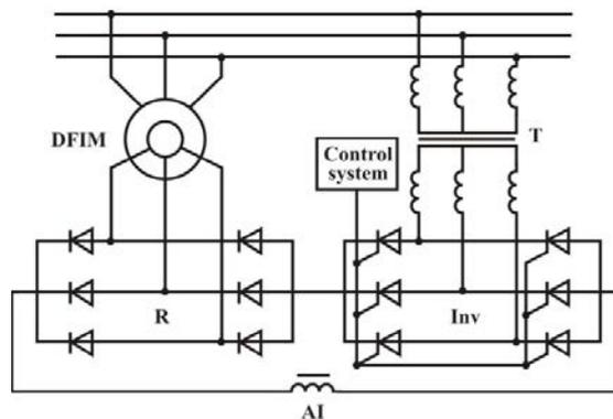
Fig. 1. An electric circuit of a centrifugal pump connected to the grid.
