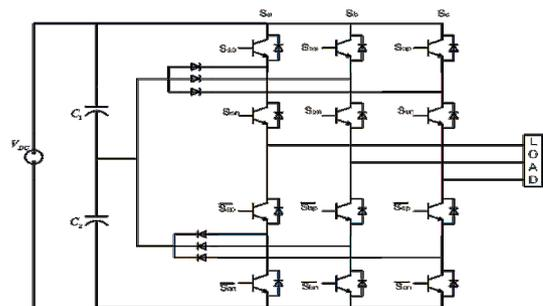
Fig. 1. NPC type Three-level Inverter Circuit
