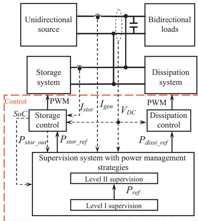
Fig. 1. System under study and supervision architecture.
