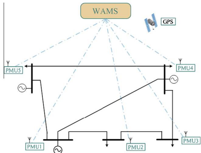
Fig. 2. The hierarchy for the wide area measurement system.
