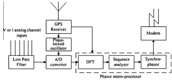
Fig. 1. A typical block diagram of PMU device.
