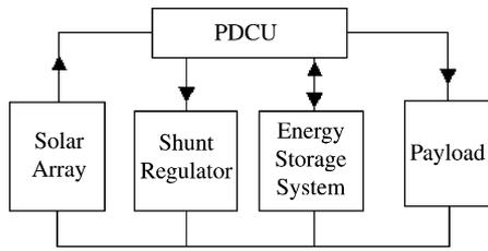
Fig. 1. Block diagram of the satellite electrical power system.
