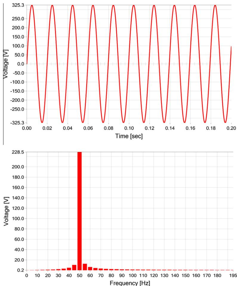
Fig. 1. Spectral leakage error ( $f_{\text{signal}} = 50.25$  Hz  $T_{\text{reg}} = 0.2\text{s} \approx 10.05$  cycles).
