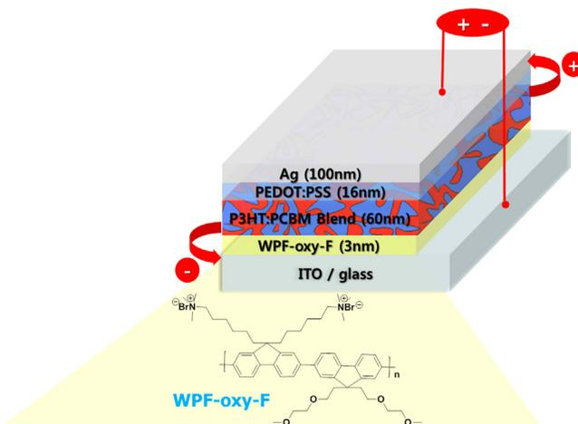
**Fig. 1.** Structure of the inverted polymer solar cell with a WPF-oxy-F layer.
