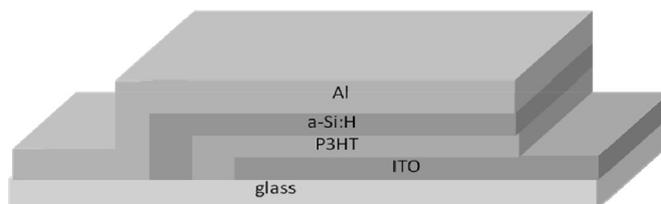
**Fig. 1.** A schematic diagram of the hybrid structure.
