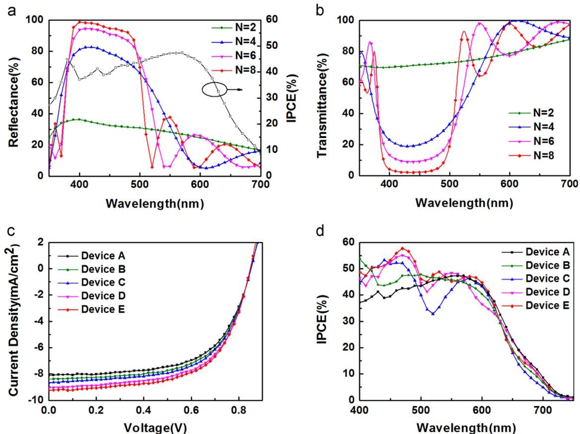
**Fig. 2.** (a) Reflectance spectra of 1DPCs and the IPCE spectrum of Device A. (b) Transmittance spectra of 1DPCs. (c)  $J$ - $V$  characteristics of Devices A–E, under  $100 \text{ mW}/\text{cm}^2$  simulated AM1.5G in ambient air. (d) IPCE characteristics of Device A–E.
