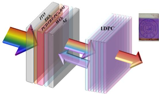
**Fig. 1.** Device architecture of STPSC with 8 pairs of 1DPC. Inset: a photograph of real STPSC with 8 pairs of 1DPC.
