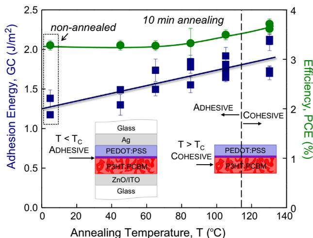
Fig. 1. The measured adhesion energy,  $G_c$  (J/m<sup>2</sup>) and efficiency, PCE (%) as a function of the 10 min annealing temperature. Insets are illustrations of the OPV device structure with either adhesive or cohesive failure.
