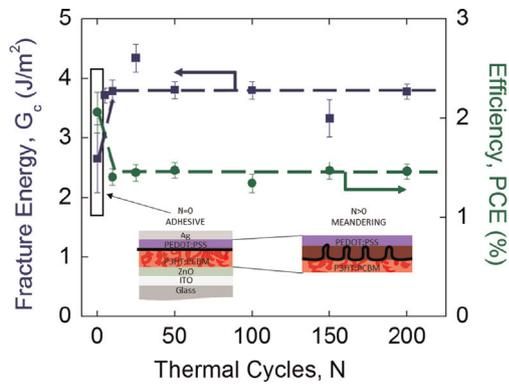
**Fig. 1.** The measured  $G_c$  ( $\text{J}/\text{m}^2$ ) and efficiency, PCE (%) as a function of thermal cycles. Insets are illustrations of the polymer solar cell device structure with either adhesive ( $N=0$ ) or meandering ( $N>0$ ) failure.
