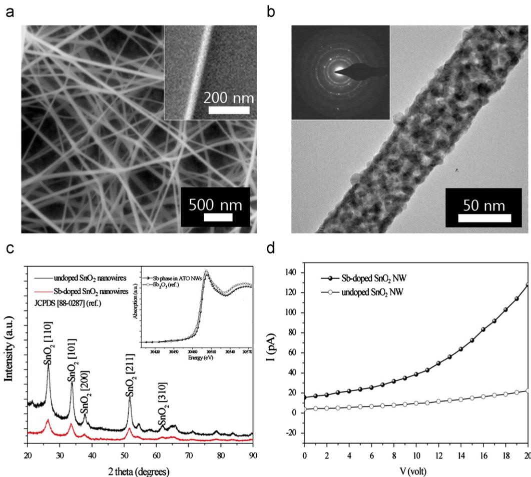
Fig. 2. (a) SEM and (b) HRTEM images (inset is selected area diffraction pattern) of ATO NWs. (c) XRD patterns of undoped  $\text{SnO}_2$  and Sb-doped  $\text{SnO}_2$  NWs; inset is XANES patterns of antimony in ATO NWs and  $\text{Sb}_2\text{O}_5$ . (d)  $I$ - $V$  curves of single undoped  $\text{SnO}_2$  nanowire and Sb-doped  $\text{SnO}_2$  nanowire.
