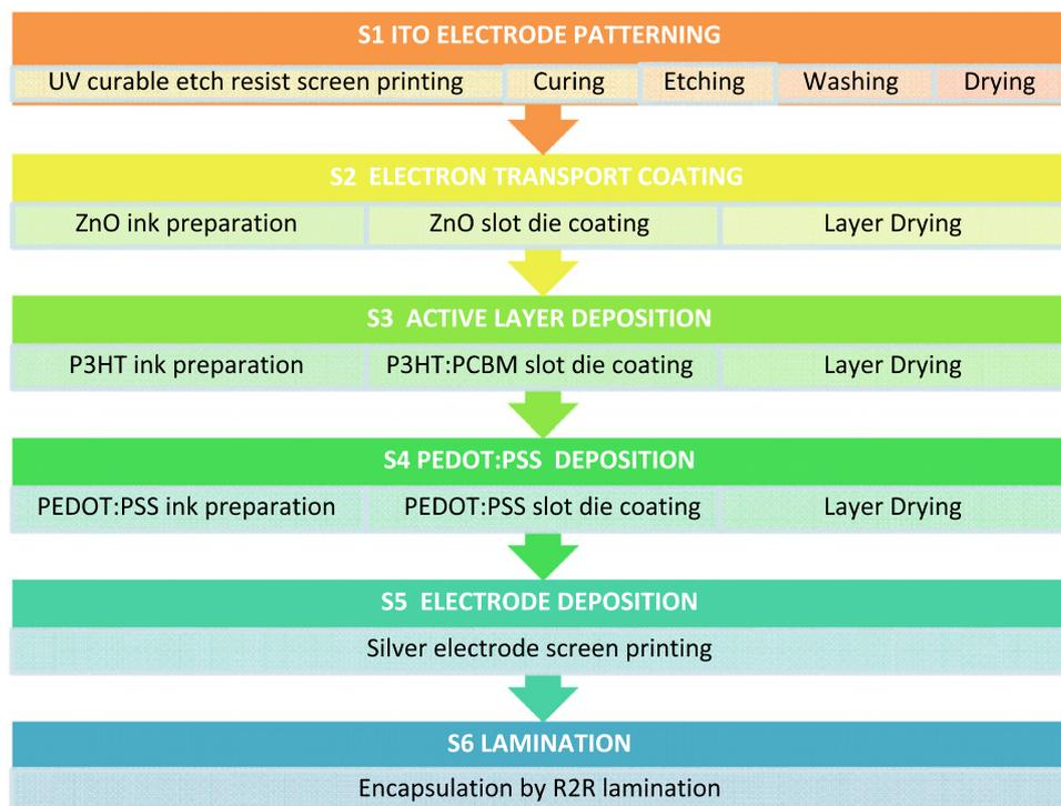
Fig. 1. Steps and substeps during the ProcessOne PV module processing.
