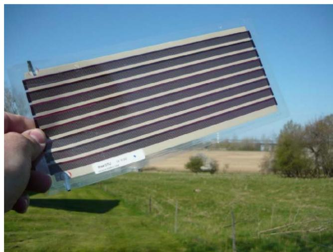
Fig. 1. The modules employed in this study as seen from the back side. The module comprises 8 serially connected devices.
