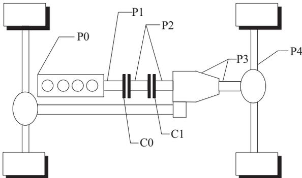
Fig. 1. Configurations of HEVs with a SEM.
