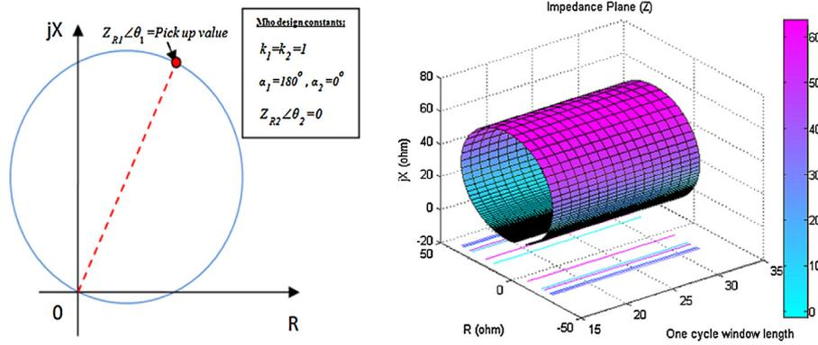
Fig. 1. Mho operation characteristic (fundamental frequency).
