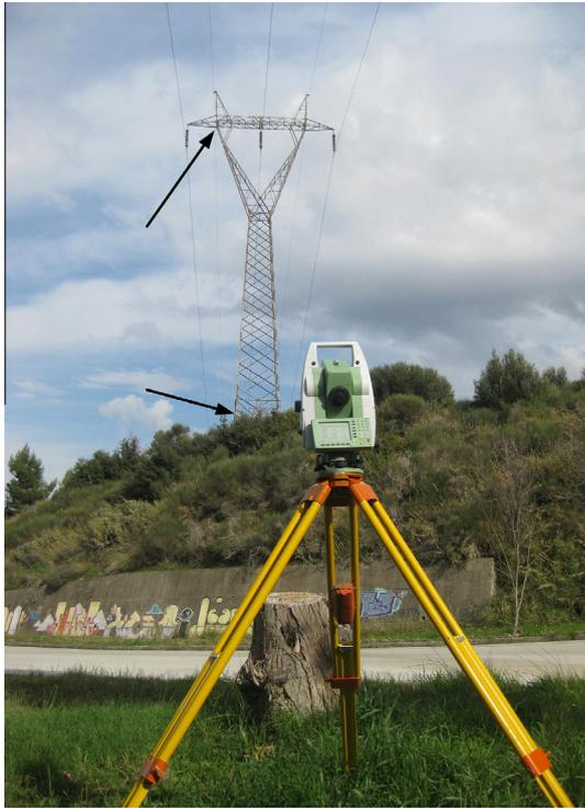
**Fig. 1.** An RTS roughly below the transmission line sighting to a reflector fixed on the upper part of the tower, marked by an arrow. A second arrow points to a second reflector (lower reflector, near the base of the tower), used to control the measurement noise.
